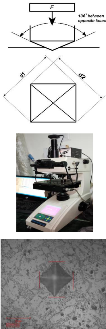
Fig. 5. Image of the Square-base Pyramid Indenter, Vicker Hardness Tester, and indentation made on the specimen after testing.
